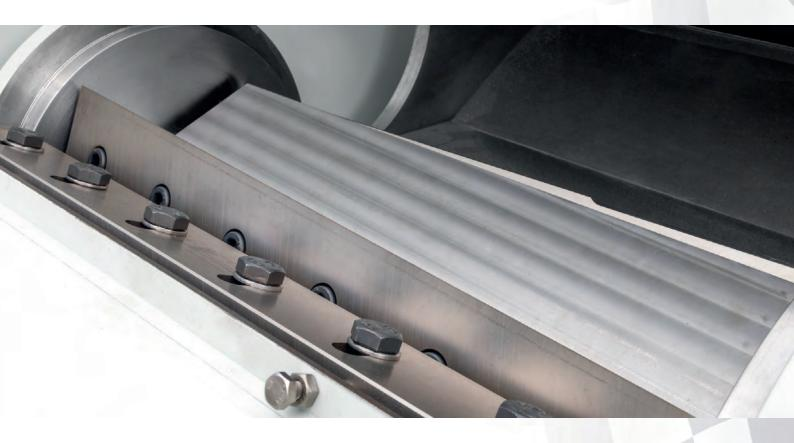
High energy-efficiency is a feature of Hellweg granulators. This is characterised by cutting rotors working according to the scissor-cut principle that have no welds, as they are produced from a solid metal blank.
