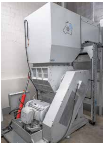
Start-up scrap and sprues that are not crushed and returned directly in production are pre-sorted and sent to large granulators in the basement. The technology of the four mills is easily accessible. They operate so quietly that they protect the people feeding the material from excessive noise.
