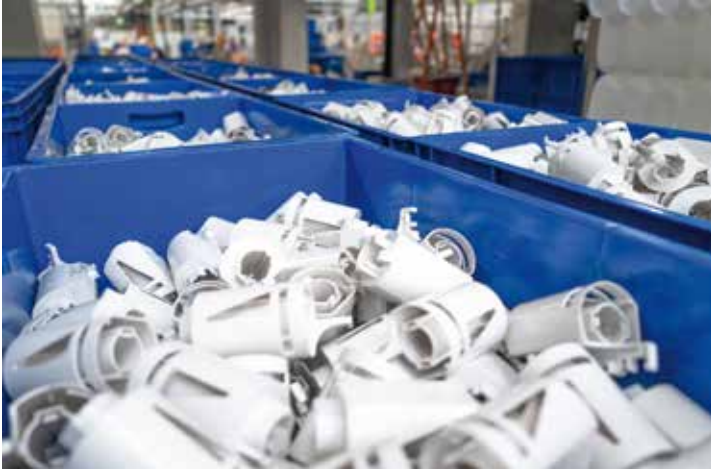
In addition to blow moulding machines for cisterns, injection moulding machines produce accessories for the cistern systems at Geberit's largest production site.
