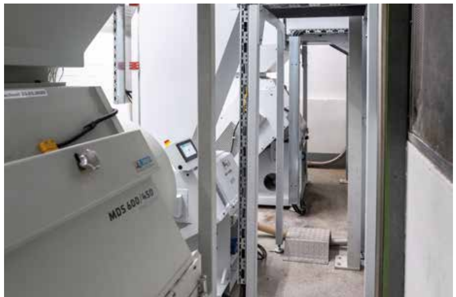
Start-up scrap and sprues that are not crushed and returned directly in production are pre-sorted and sent to large granulators in the basement. The technology of the four mills is easily accessible. They operate so quietly that they protect the people feeding the material from excessive noise.
